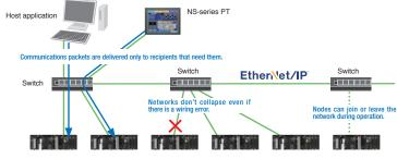
Star topology using Ethernet switch technology
